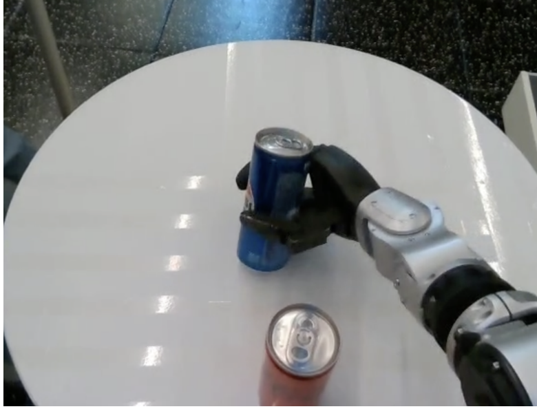
Figure 4 Example of a real-robot pick-and-place task using the learned VLA policy. The Unitree G1, equipped with a Dex-3 hand, grasps the target can from the tabletop using egocentric visual observations.
